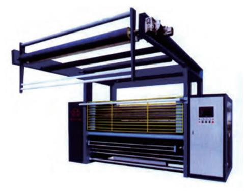
SMA168, 24 rollers, Its suitable for raising mink blanket, wool, Short hair velvet surface such as heavy thick fabric SMA168, 36 rollers, its suitable for cotton, wool fabric and blended fabric of warp knitting coral fleece, weft coral velvet, warp knitting cloth, flannelette, spandex velvet, faux suede, base fabric of Nubuck leather, such as light thin fabrics
